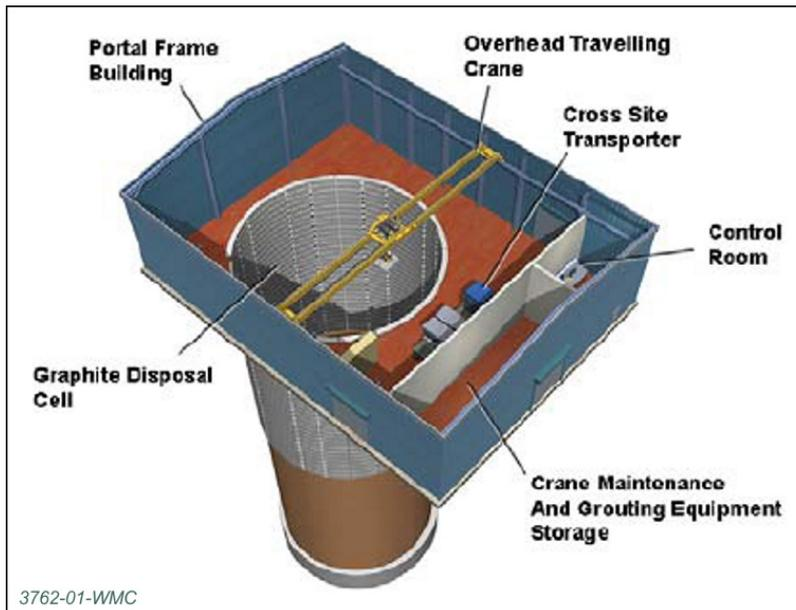
The silo would be constructed from the surface with concrete segment walls forming part of the multi-barrier containment along with a substantial reinforced concrete base slab. Cement-encapsulated waste in boxes would be stacked in the silo with the remaining gaps grouted to create a monolith within the disposal cell.
